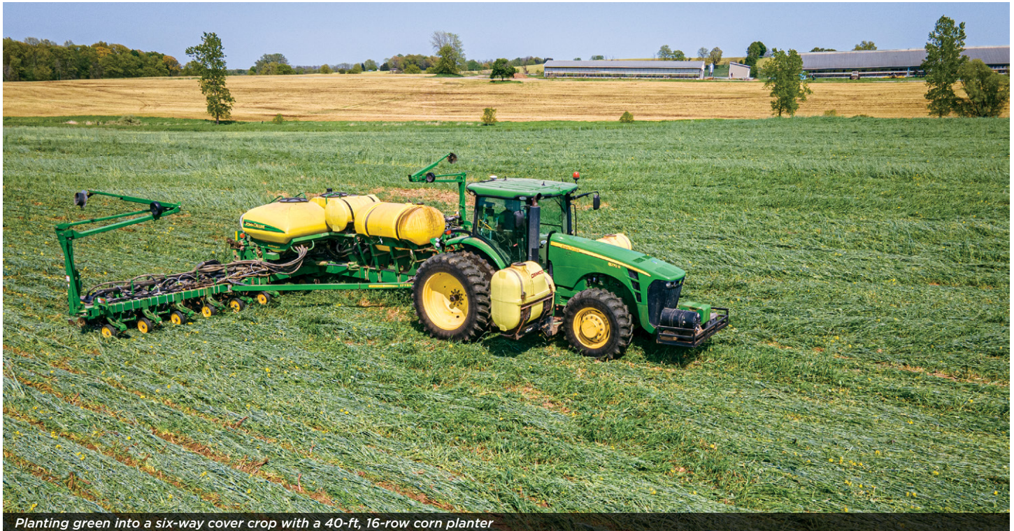
Planting green into a six-way cover crop with a 40-ft, 16-row corn planter
